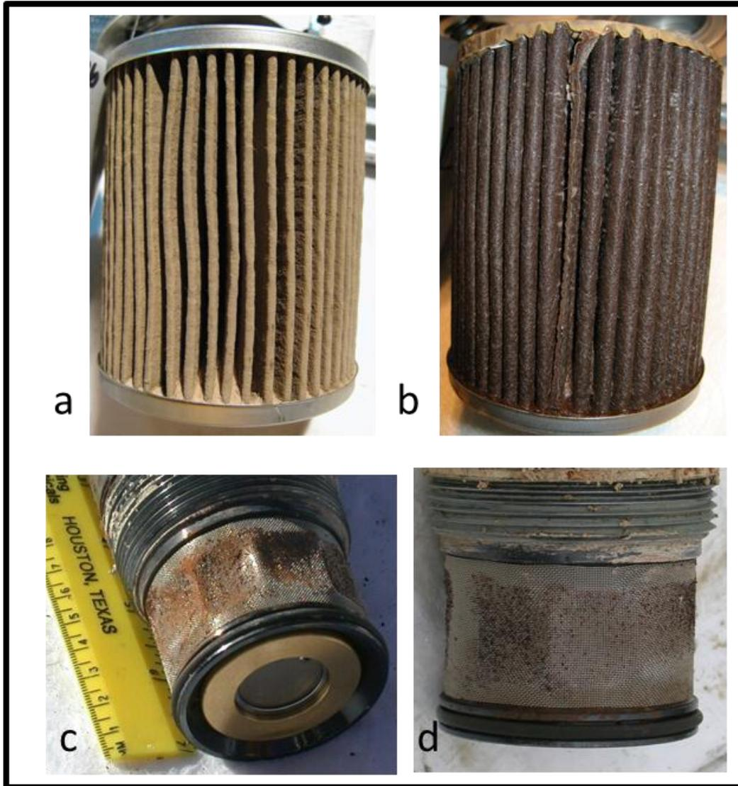
a) Unfouled dispenser filter element from 87 RON gasoline retail site fuel dispenser; b) heavily fouled dispenser filter element from 87 RON gasoline retail site fuel dispenser; c) 87 RON gasoline retail system leak detector screen that has partially imploded due to accumulated rust particles on its surface; d) 87 RON gasoline retail system leak detector screen with minor accumulation of rust particles.
